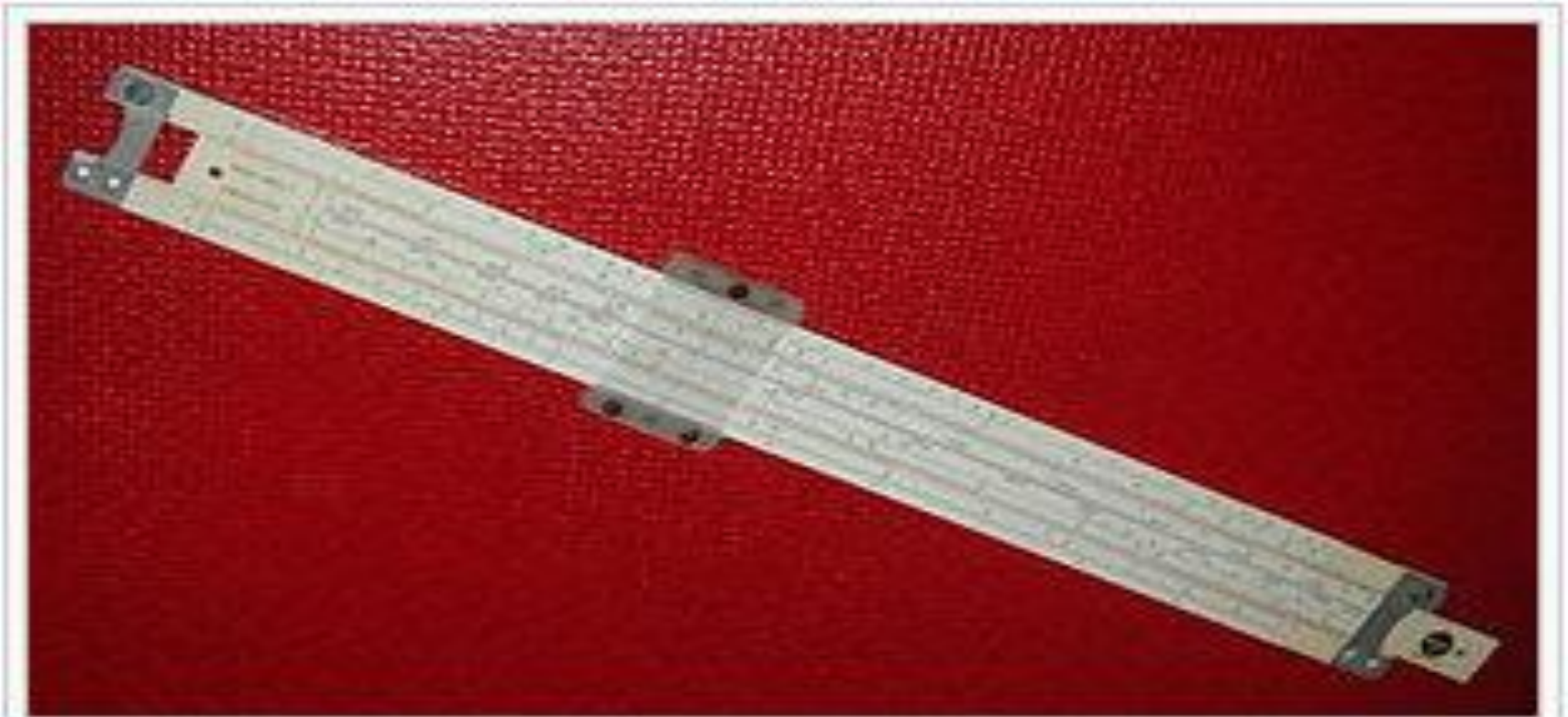
A typical ten-inch student slide rule (Pickett N902-T simplex trig).
